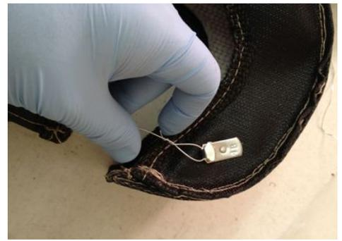
Now install the blanket around the exhaust side of the turbocharger and snug it down by hooking your twisted safety wire around the opposite hook on the turbo blanket.
