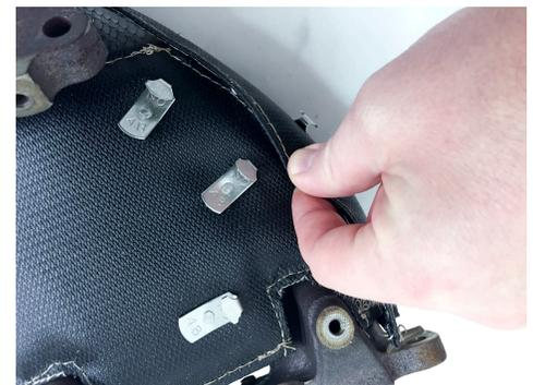
You will need 7 lengths of wire about 3-5 inches long, we suggest making a loop in one end of each of the wires to make lacing the blanket easier.(figure 4)
